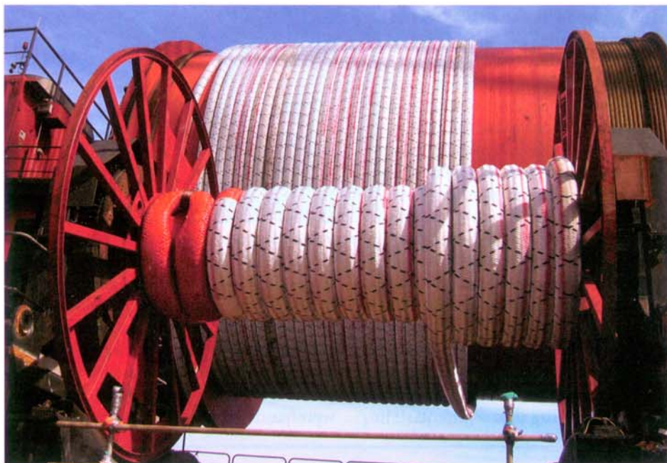
Figure 1. Mooring Line Deployment Winch (MLDW) is shown onboard Balder . (Images courtesy of Heerema)
