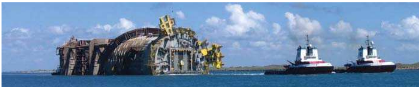
The Perdido spar being towed to position in the Gulf of Mexico.
