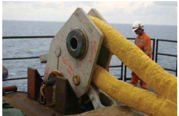
(Above) Connecting sections together with H-links. (Below) Handling chain.
