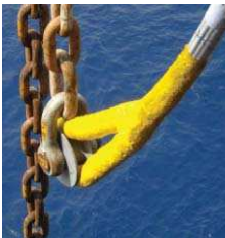
View of both chain and polyester mooring line.
