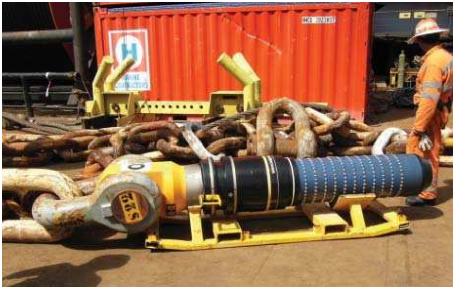
Perdido First Subsea male SMC with mooring chain attached.
