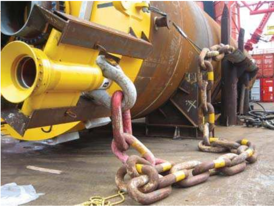
Perdido First Subsea female SMC with ground chain attached to pile.
